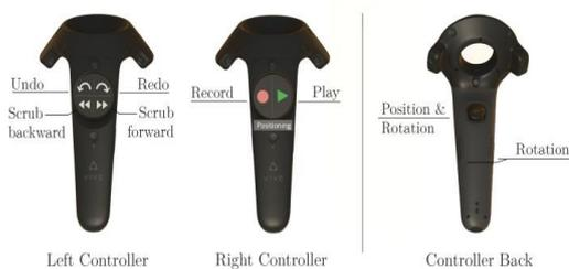
Fig.3 Left and Right Controller for the layout of the function. The functions mentioned on front side is the same as backside.
